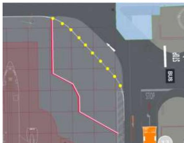
Fig. 2 – Detail: placement of delineator posts and road/ESA markings
